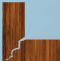
Cracking Caused By Groove Cutting or L - Shaped Cutting.
